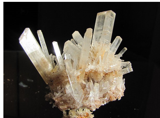
Gypsum, or hydrated calcium sulfate, is softer and less dense than anhydrite, or anhydrous calcium sulfate.
